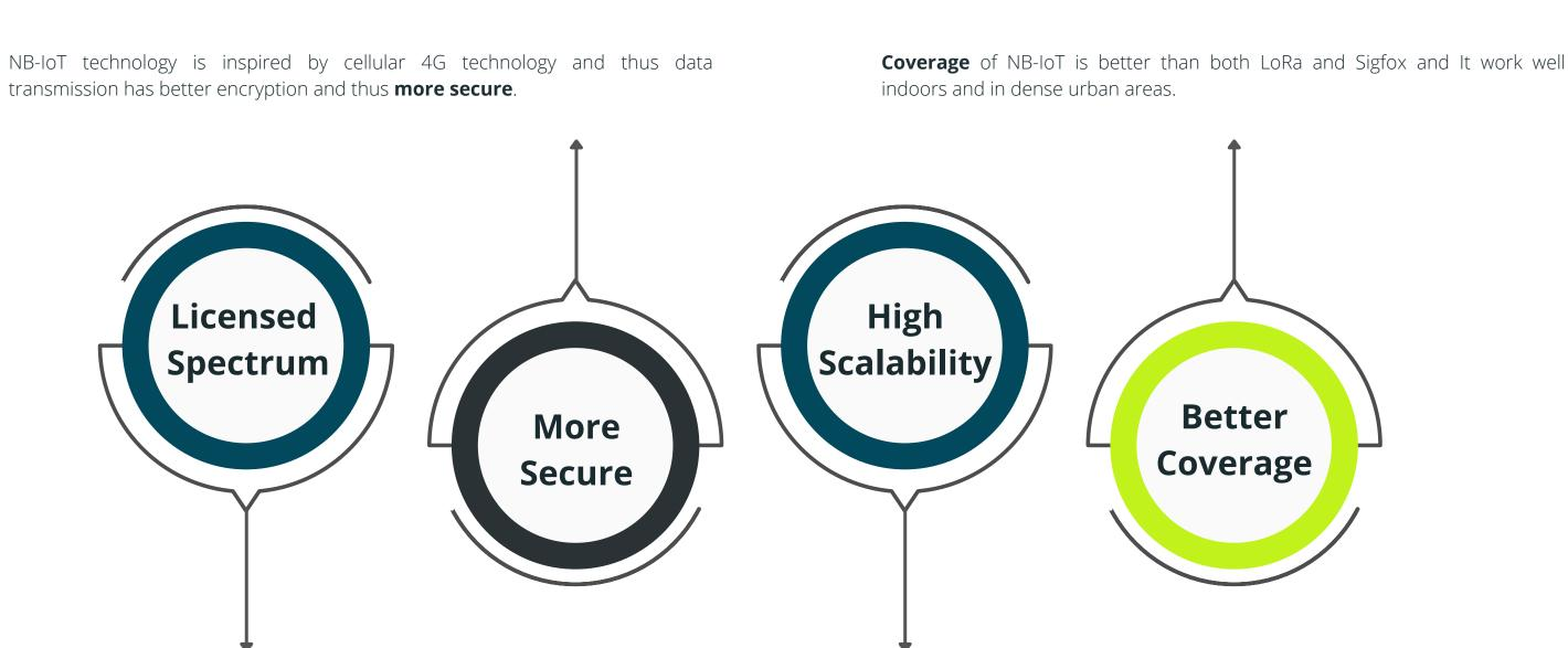
Sigfox and LoRa employ unlicensed spectra and asynchronous communication protocols whereas NB-IoT employs a licensed spectrum and an LTE-based synchronous protocol, which are optimal for quality of service at the expense of cost.
