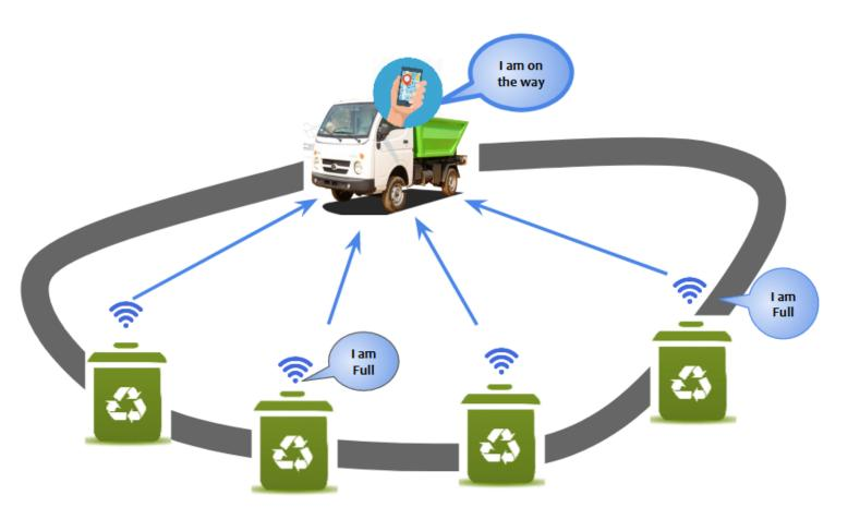
**Smart Garbage Management System:** A smart garbage management system contains sensors attached with the garbage bins which monitor the garbage loading level. Once the garbage bin is fully loaded, the attached garbage sensor transmits the data to the garbage collector along with the location address of the bin. The garbage data is only communicated once the bin is fully, thus NB-IoT helps in cost reduction for the process too.
