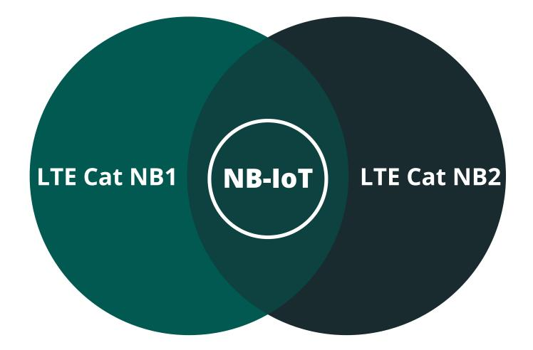
LTE Cat NB1 refers to IoT devices based on the NB-IoT protocol standardized in the 3GPP Release 13 specification. It is a wireless cellular low-power wide-area connectivity protocol for IoT massive machine-type communications.
